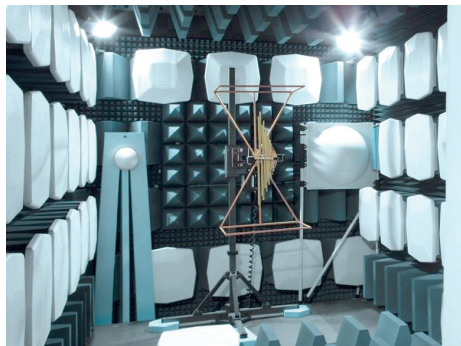
3 m FAR chamber, test volume \varnothing 0.9 x 1.2 m, max. weight 500 kg
